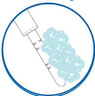
**Why** – Deposits on the probe can build-up over time on the electrode portion and the vent hole. This can cause erratic readings and issues calibrating.
