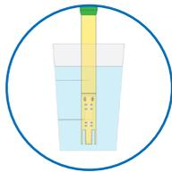
**Why** – Incomplete submersion can cause erratic and/or inaccurate readings.
