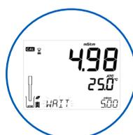
**Why** – Even if a probe has integrated temperature compensation, it takes time for the probe to reach thermal equilibrium.
